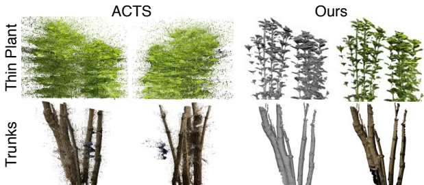
Figure 6: Comparison of our technique to the ACTS software [41]. For our algorithm, we show our resulting mesh with and without texture. Since ACTS produces point clouds, we show these from two different viewpoints.
